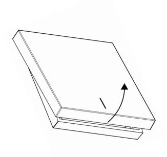
2. Attach the plate to the wall, ensuring that it is oriented with the correct side facing upwards. Secure it by screwing it into place. After securing the plate, reattach the front plate to complete the installation.
